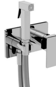
PROFILI Plus douche kit with shut-off ✓ Minimum 0.5 bar ✓ Height 60mm ✓ Width 137mm ✓ Hot & Cold mixer ✓ With handset & hose
